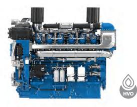
Number of cylinders Bore and stroke (mm) Total displacement (L) Cylinders Engine rotation Idle speed Flywheel Flywheel housing 12 180 x 215 65.6 12V counter clockwise 600 21" SAE 00
