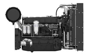
$\begin{array}{lll} \text{Bore x Stroke (mm)} & 105 \times 130 \\ \text{Displacement (L)} & 9.7 \\ \text{N° of Cylinders} & 6 \\ \text{Cylinders Arrangement} & \text{In line} \end{array}$
