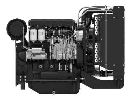
Bore x Stroke (mm)105 x 130Displacement (L)4.5N° of Cylinders4Cylinders ArrangementIn lineFuel SystemMechanical PumpGovernor (Gov.)MechanicalAspiration (Asp.)Turbocharger
