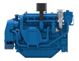
Number of cylinders Bore and stroke (mm) Total displacement (L) Compression ratio Engine rotation Idle speed (rpm) Flywheel Flywheel housing 6 in line 105 X 130 6.75 18/1 counter clockwise 650 SAE 3 SAE 11.5"
