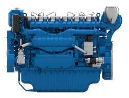
Number of cylinders Bore and stroke (mm) Total displacement (L) Compression ratio Engine rotation Idle speed Flywheel Flywheel housing 6 in line 150 X 185 19.6 15/1 counter clockwise 650 SAE 1 SAE 14"
