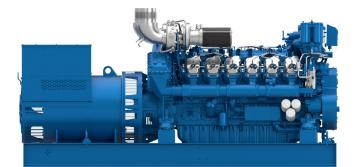
Number of cylinders Bore and stroke (mm) Total displacement (L) Compression ratio Engine rotation Idle speed Flywheel Flywheel housing 12V @ 90 126 X 185 39.2 15/1 counter clockwise 650 SAE 0 SAE 18"
