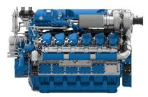
Number of cylinders Bore and stroke (mm) Total displacement (L) Compression ratio Engine rotation Idle speed Flywheel Flywheel housing 12V @ 90 150 X 150 31.8 15/1 counter clockwise 650 SAE 0 SAE 18"
