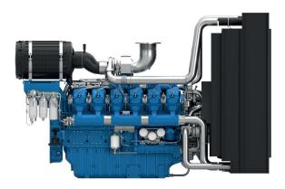
Bore & Stroke (mm)150 x 150Displacement (L)31.8N° of Cylinders12Cylinders ArrangementAt VeeFuel SystemMechanicalGovernor (Gov.)ElectronicAspiration (Asp.)T/A-A
