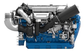
Number of cylinders Bore and stroke (mm) Total displacement (L) Engine rotation Idle speed Flywheel housing Flywheel 6 in line 127 X 165 12.5 counter clockwise 700 SAE 1 SAE 14"
