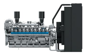
Bore & Stroke (mm) Displacement (L) N° of Cylinders Cylinders Arrangement Fuel System Governor (Gov.) Aspiration (Asp.) 150 x 185 65.4 20 At Vee High Pressure Common Rail ECU Turbocharged and Aftercooled
