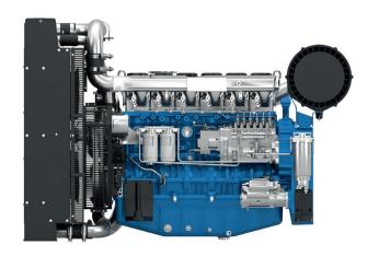
$\begin{array}{lll} \text{Bore \& Stroke (mm)} & 127 \times 165 \\ \text{Displacement (L)} & 12.54 \\ \text{N° of Cylinders} & 6 \\ \text{Cylinders Arrangement} & \text{In line} \\ \end{array}$
